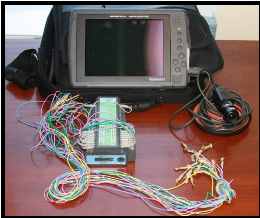
Portable EEG Monitoring Equipment
